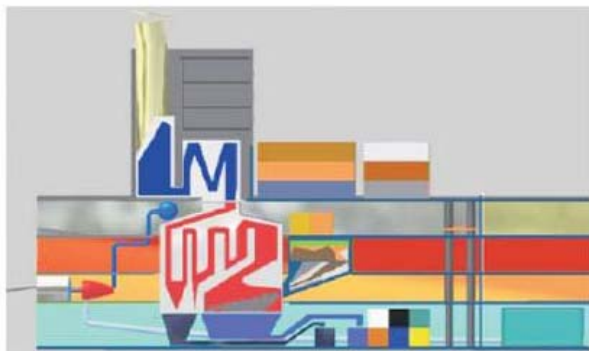
Boiler, Flue Gas Treatment and fuel handling Systems
